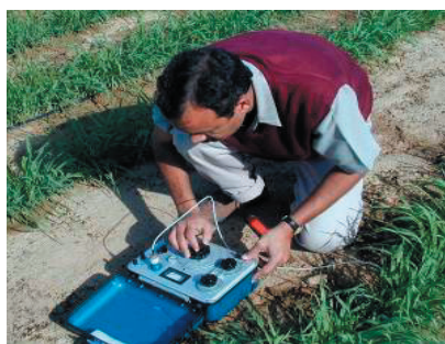
Figure 25b. Salinity monitoring using salinity bridge in barley field.
