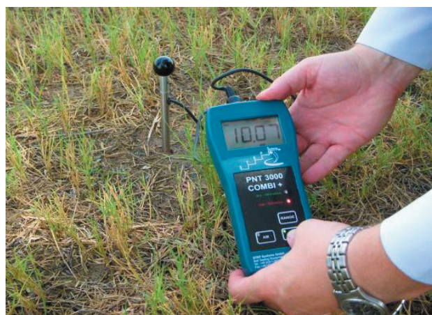
Figure 23b. In-situ salinity probe.
