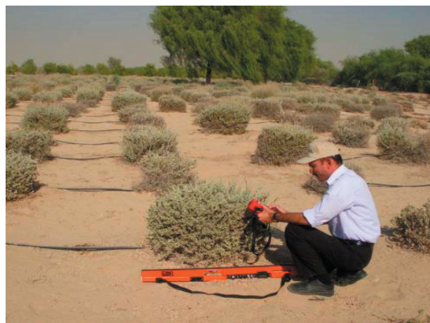
Figure 21b. EM 38 in Atriplex field ICBA Station (horizontal mode).
