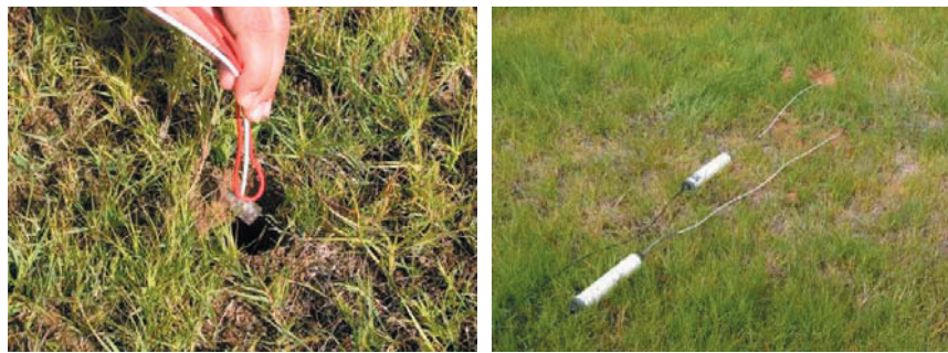
Sensor placement in the grass rootzone Buried sensors connected to smart interface.
