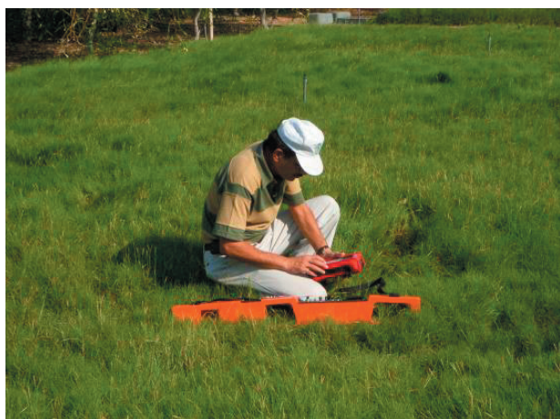
Figure 21a. EM38 in grass field – ICBA Station (vertical mode).
